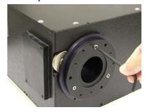
**3.** Loosen set screw with 3/32" hex wrench. **4.** Loosen set screw.
